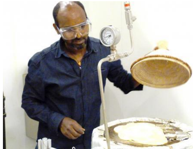
The inventor Asfafaw Tesfay in the process of baking injeras on his solar powered oven. (Photo: Dag Håkon Haneberg)
